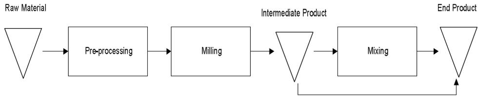
**Figure 1.** Flour milling production process
